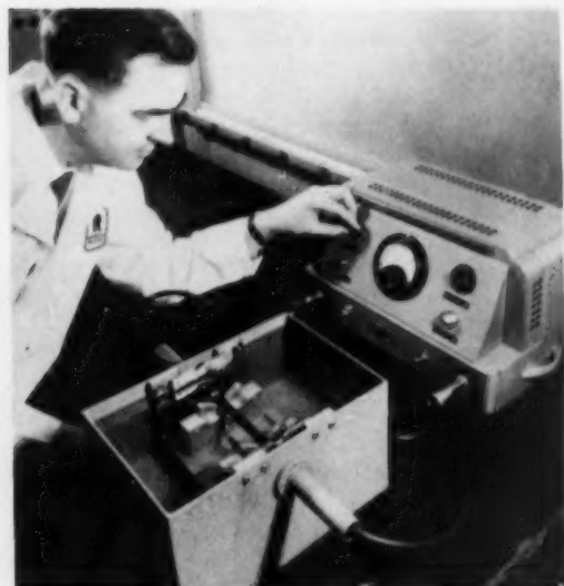
Fig. 2—Composite unit includes universal test tank and cradle for small parts, electronic transmitter and receiver, and transducers.
